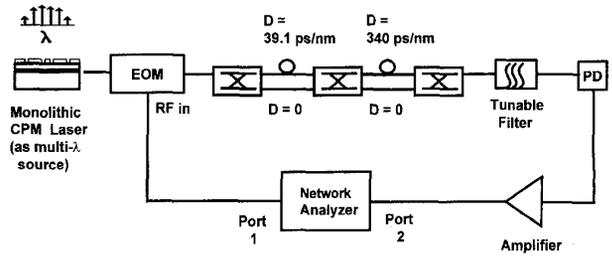
Fig. 3. Experimental setup for characterizing the relative RF phases of the MWOCFAA with a 2-bit PDM.
