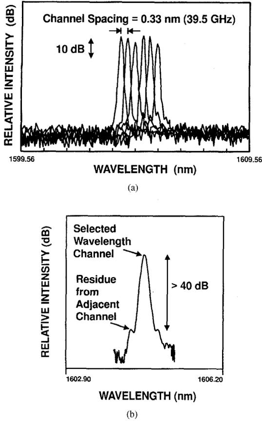
Fig. 2. (a) Six wavelength channels extracted from a 39.5 GHz monolithic mode-locked semiconductor laser by using a double-grating demultiplexer. (b) Side-mode-suppression-ratio for each wavelength channel is greater than 40 dB.
