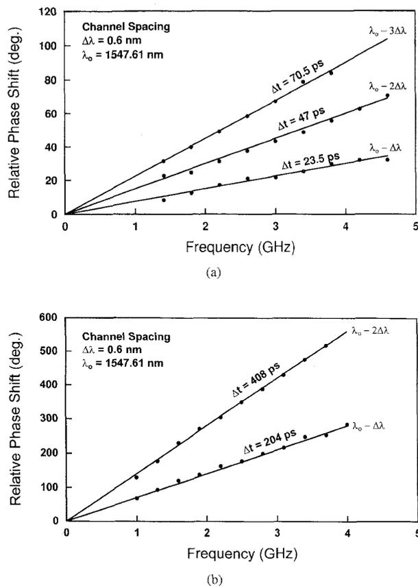
Fig. 4. Relative RF phase shift versus frequency for various channels relative to the reference channel at  $\lambda_0 = 1547.61$  nm. The total dispersions of the fibers are (a) 39.1 ps/nm, and (b) 340 ps/nm.
