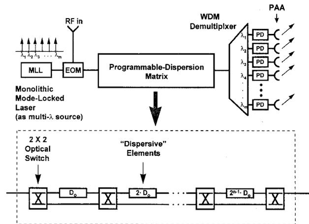
Fig. 1. Schematic diagram of the proposed MWOCPAA architecture using a multiwavelength laser and a programmable dispersion matrix.
